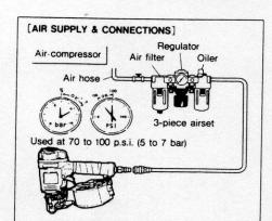
FITTINGS: Install a male plug on the tool which is free flowing and which will release air pressure from the tool when disconnected from the supply source.
