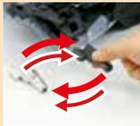
By using two different sizes of nose contacts, HN65 can drive nails with shank diameters from 2.1 mm to 3.3mm
