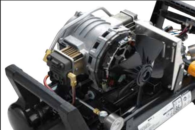
It has a dual-cylinder that takes air through 2 stages to make the air pressed up to 34bar by using the DC brushless motor. This compressed air provides power to the nailer and can drive through wood, concrete and steel. Inverter control allows it to operate in a low voltage situation from 140V up to 265V.
