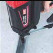
Easy to position in the corner with contact nose
