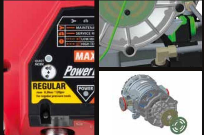
It has a "Floating Motor" mechanism. This design mounts the motor on a flexible rubber support and together with a silent filter this lessens the operating sound of the compressor.
